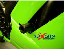
5. Put one drop of blue thread locker on the end of the thread mount right side puck to the offset using 99-HB-SH10150045 Socket Cap 10 X 1.5 X 45. Torque down to 30 to 32 foot lbs.
