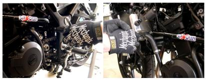
7. Mount the right side rail using(99-HN-LN9/1618-F&R) 9/16 18 Pitch Hex Flange Serrated Nuts and torque down to 32ft lbs.
