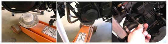
6. Loosely mount the left side rail passing the (99-HR-TH3/8-16 x6 11/16-R)9/16 X 160 welded threaded rodin the rear through the Shogun rail towards the right side of the bike. Use the (99-HR-TH3/8-16x9 15/16-F) 9/16X 245 welded threaded rod in the front. Pass it through the Shogun rail towards the right side of the bike. When installing the front rod lightly press down on the radiator hose so the bolt can pass.
