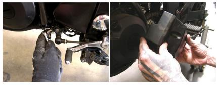
4. Loosen front and rear engine through studs. Do not remove studs until after step 5.
