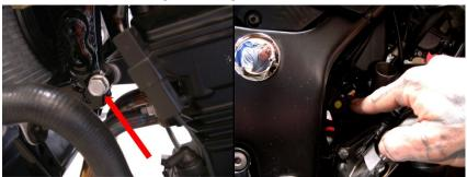
5. Make sure the vehicle is in a fixed secure position. With a standard floor jack support the engine enough to remove engine studs. To help prevent scratching of any kind or damage to the bike when lifting we use a small piece of soft wood or a plastic puck on the jack pad. With jack secure and in place remove each front and rear stock engine studs.
