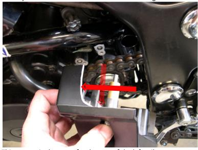
This cut out is clearance for the rear of the left rail.
