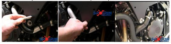
6. Remove the bodywork and double check location of spot mark the tool has created.
