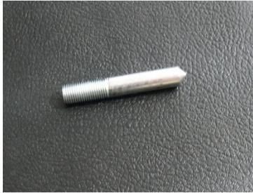
With the body removed, thread in by hand your spot tool. Make sure you have the spot tool screwed in enough to clear the body on the inside.
