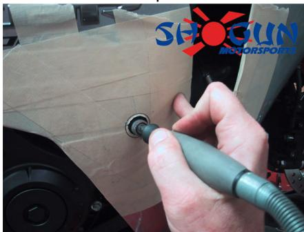
10. Mend the inner heat shield back to the panel and trim to match hole diameter. Tip: We used high temp 3M adhesive.
