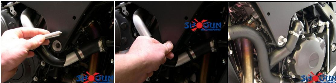
6. Remove the bodywork and double check location of spot mark the tool has created.
