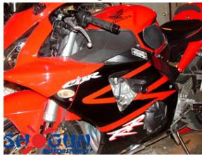
2. Remove right side bolt. Mount right side puck with (99-HB-SH10125080) Socket Cap 10 X 1.25 X 80 Main Engine Stud and torque down.
