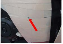
7. A pencil was then used to draw our diameter of desired shaped hole. A flexible hole template can also be used for the same purpose. Place the hole template on center of the pilot hole (or spot tool) and draw your desired diameter.
