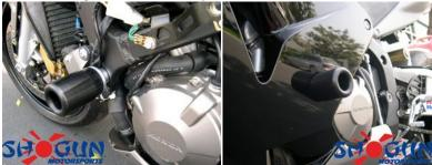
10. Remove right side bolt. Loosen pinch bolt mount right side puck with (99-HB-SH121250120) Socket Cap 12 X 1.25 X 120 Main Engine Stud and torque down, then pinch bolt.
