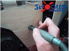
9. Remove left side bolt. Mount left side puck with (99-HB-SH121250120) Socket Cap 12 X 1.25 X 120 Main Engine Stud and torque down.
