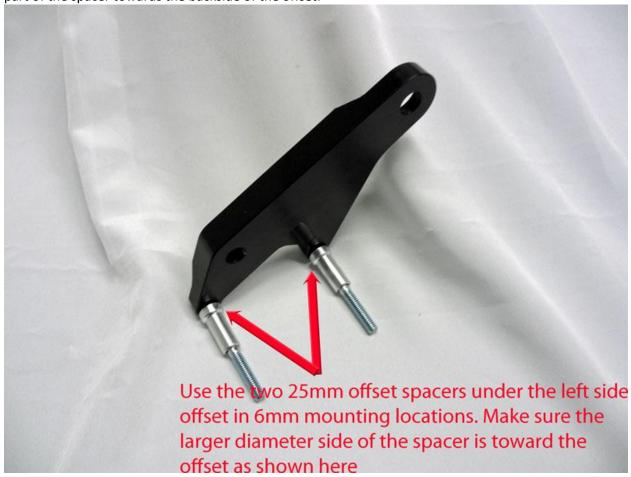
4. Mount left side offset (LOOSELY) by hand using all 3 bolts. Tighten both 6 X 1.00 X 60 (99-HB-SH0610060) socket cap bolts (FIRST) then main OEM engine stud. Check service manual for 6mm and main engine stud OEM torque specs.
