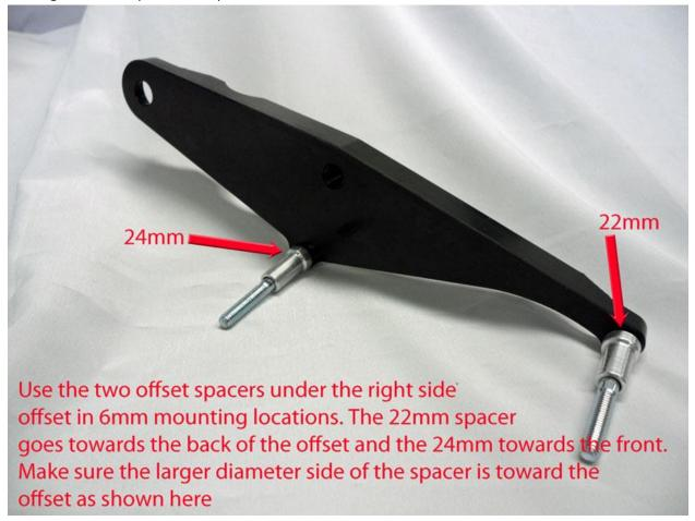
6. Mount right side offset (LOOSELY) by hand using all 3 bolts. Tighten both 6 X 1.00 X 60 (99-HB-SH0610060) socket cap bolts (FIRST) then main OEM engine stud. Check service manual for 6mm and main engine stud OEM torque specs.
