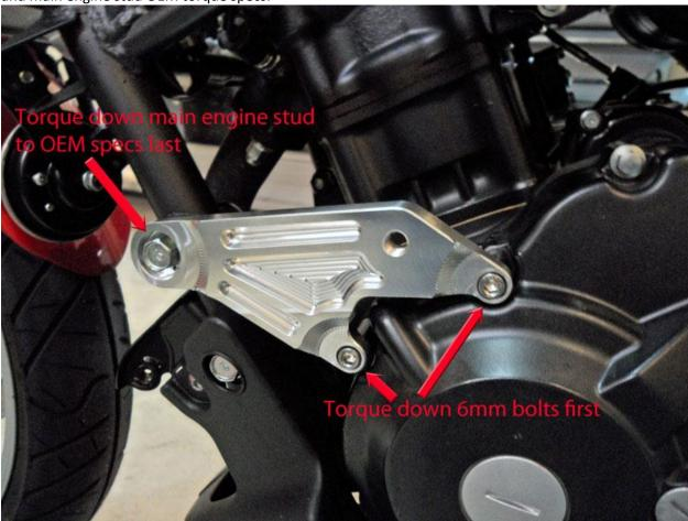
5. Before right side offset is installed pre assemble the offset using two 6 X 1.00 X 60 (99-HB-SH0610060) socket cap bolts and two 22mm (428-9107) & 24mm (428-9106) offset spacers with the larger diameter part of the spacer towards the backside of the offset.
