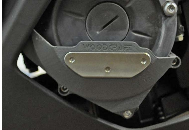
3) Install the Woodcraft cover using the included mounting hardware. Torque for these mounting bolts is about 7 ft-lbs.
