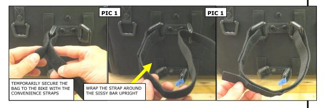
Refer to **PICS 2 and 3**. Use the included Straps and "D-rings" to secure the bag to at least four (4) secure points on the motorcycle (two in the front and two in the rear).
