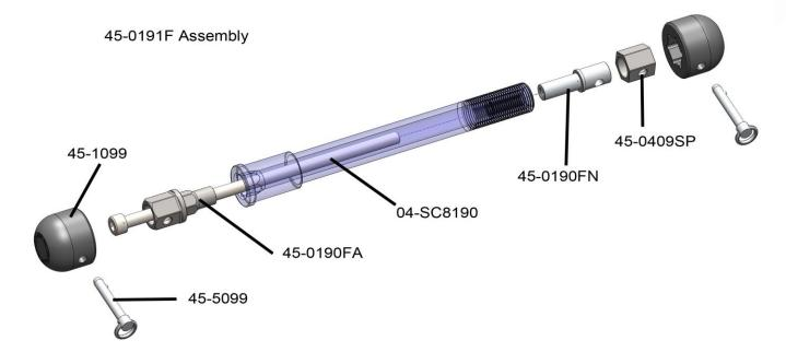
A note for racers: If your tech inspector wants you to safety wire these (most will not) then you need to orient the pins so that the safety wire acts to pull the pin into the puck.
