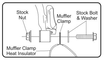
Standing at the back of the motorcycle, check for proper alignment of the muffler and adjust if necessary.
