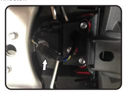
While securely supporting the stock fender assembly, remove the four bolts securing the fender assembly to the frame. Carefully remove the stock fender assembly making sure not to damage the connectors in the process.
