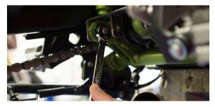
10. Slide S1R muffler onto TBR Slip Tube.
