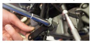
Loosely install the TBR slip tube and barrel clamp to the TBR headers.
