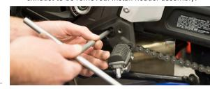
Loosely install TBR headers using the OEM flange nuts.
