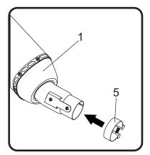
Install (No. 1) *Muffler,* tailpipe over the stock header outlet. Align and secure to the stock muffler mount using the stock bolt, washer, (No. 4) 5X25SPC, aluminum spacer and nut.
